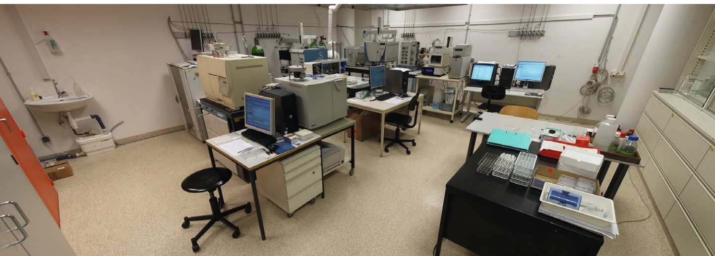
Overview of SILVER laboratory with five isotope ratio mass spectrometers allowing bulk and compound-specific analysis of hydrogen, carbon, nitrogen and oxygen in biological and environmental samples
