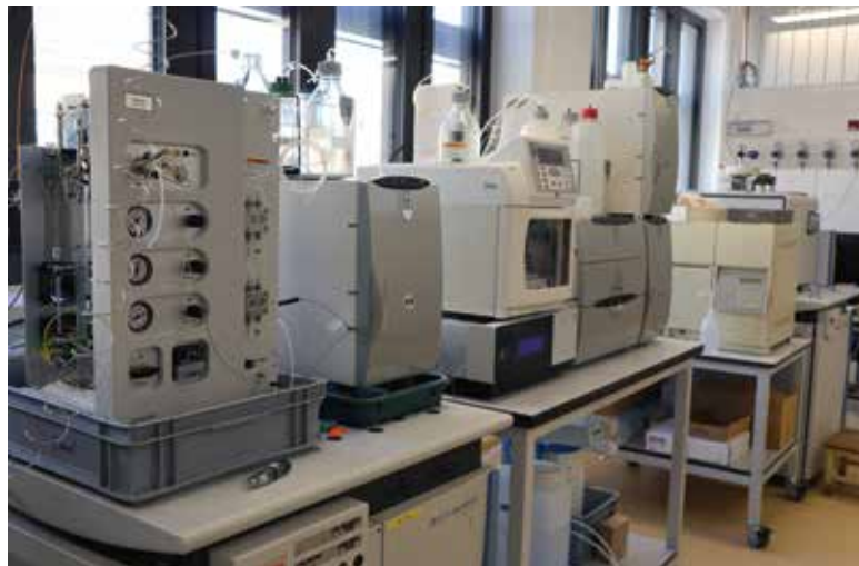
A suite of isotope ratio mass spectrometers (IRMS) for bulk and compound-specific analysis of hydrogen, carbon, nitrogen and oxygen in environmental samples. Credit: Pamela Nölleke
