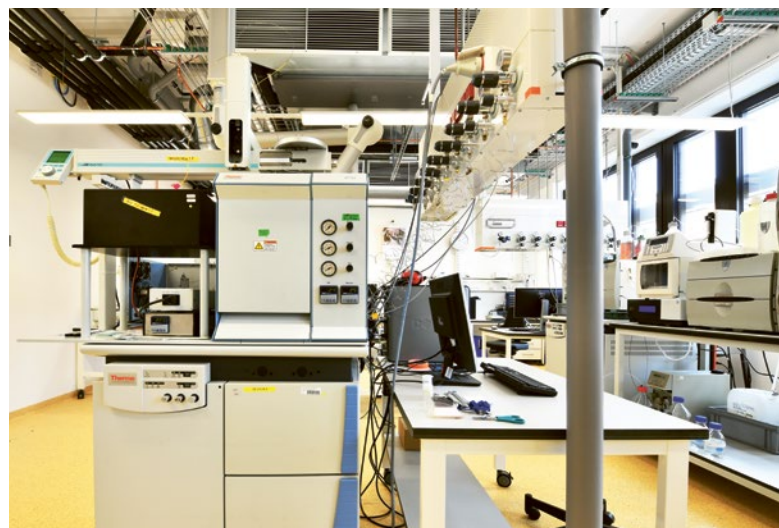
A suite of isotope ratio mass spectrometers (IRMS) for bulk and compound-specific analysis of hydrogen, carbon, nitrogen and oxygen in environmental samples. Credit: Reinhold Leitner
